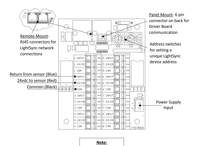
Maximum power draw per module is 800mA@24vdc
